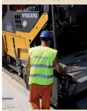
External EPM control panels at both sides of the screed.
